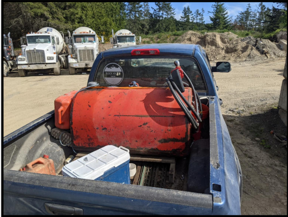
Photo 19 – Tidy tank found within Site Supervisors truck, used for fueling equipment onsite when required.
