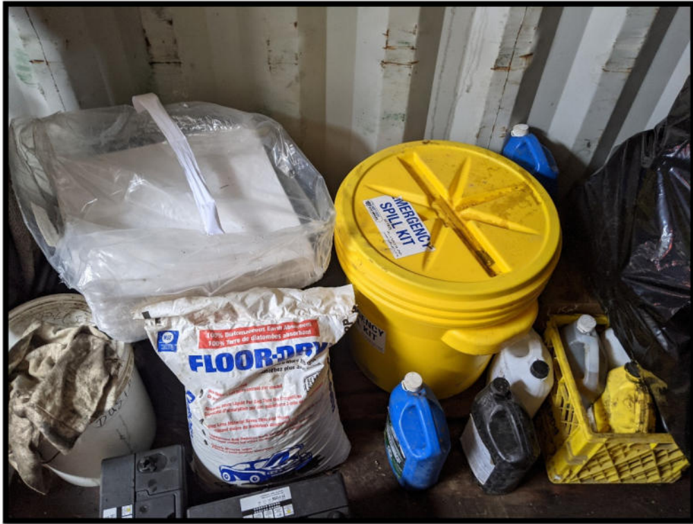
Photo 17 – Spill kit within hydrocarbon storage area.
