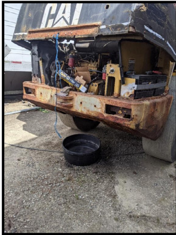
Photo 14 – Drip trays were noted under most stationary vehicles at time of inspection.
