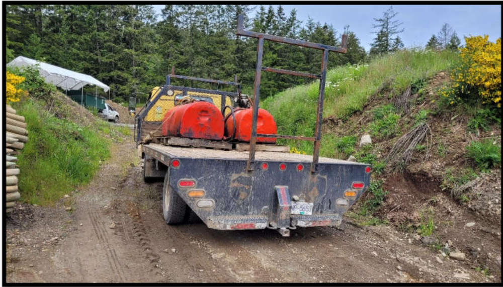
Photo 17 – Tidy tanks aboard flat bed truck, used for fueling equipment onsite.
