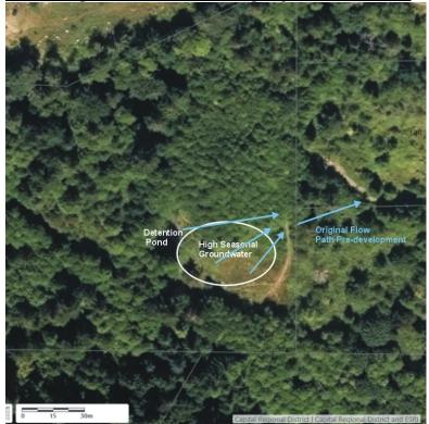
In addition to the IT Bylaw 355 purpose of minimal disturbance to existing surface and groundwater flows, the design for storm water drainage, and the drainage to enable construction in the area with high seasonal water table, is intended to restore flow patterns towards Ganges Creek which are already disturbed.
