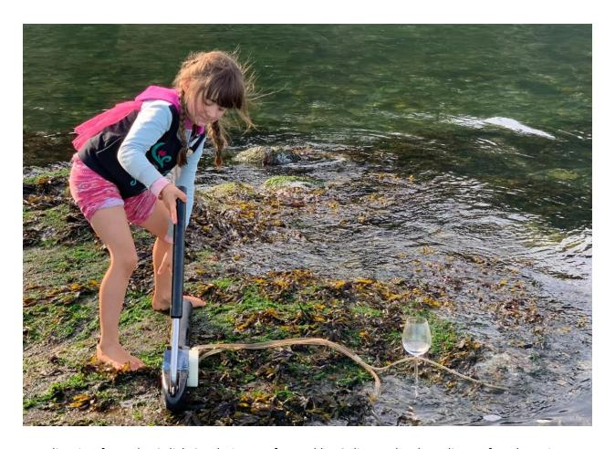
Desalination from the Salish Sea being performed by Galiano Islander Edie Keefer, then six years old. The motorized version of this hand-operated desalinator can produce 100 liters per day, drawing 50 watts of 12 volt power. The brine discharge is only 10% more salty than the feed seawater.
