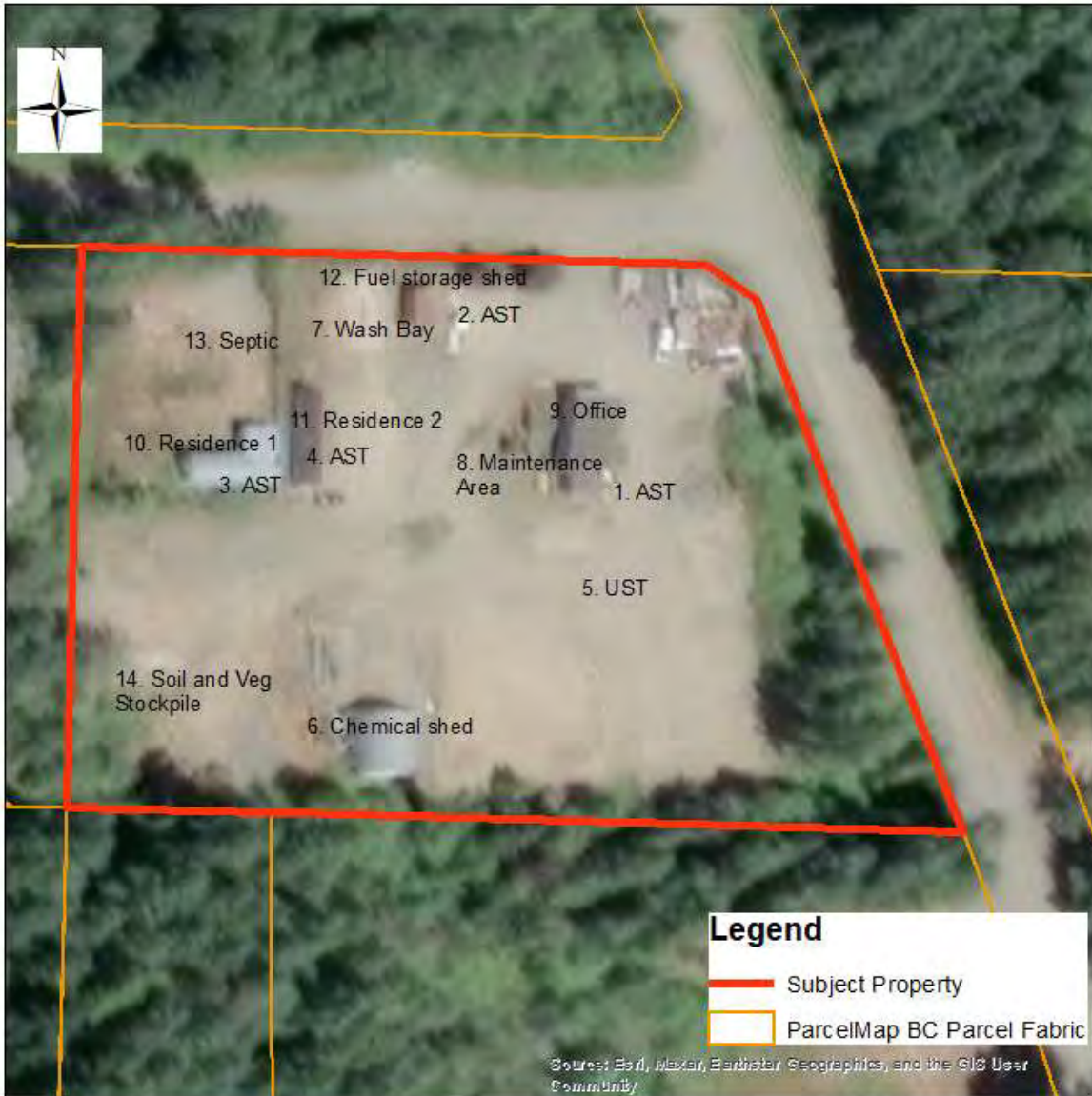
Figure 4. Location of APECs on the subject property and adjacent properties. APECs are listed in Table 1 (Section 6.0).
