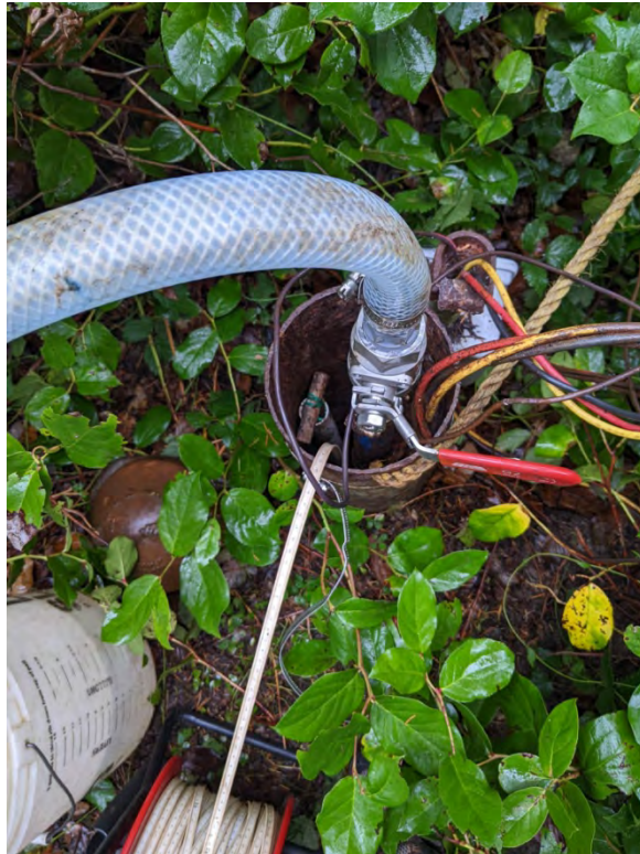
Photo 5. Emcon well head during step test with water level measurement in progress.
