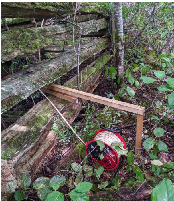
Photo 2. Wooden enclosure around the Dug Well with depth to water measurement in progress.
