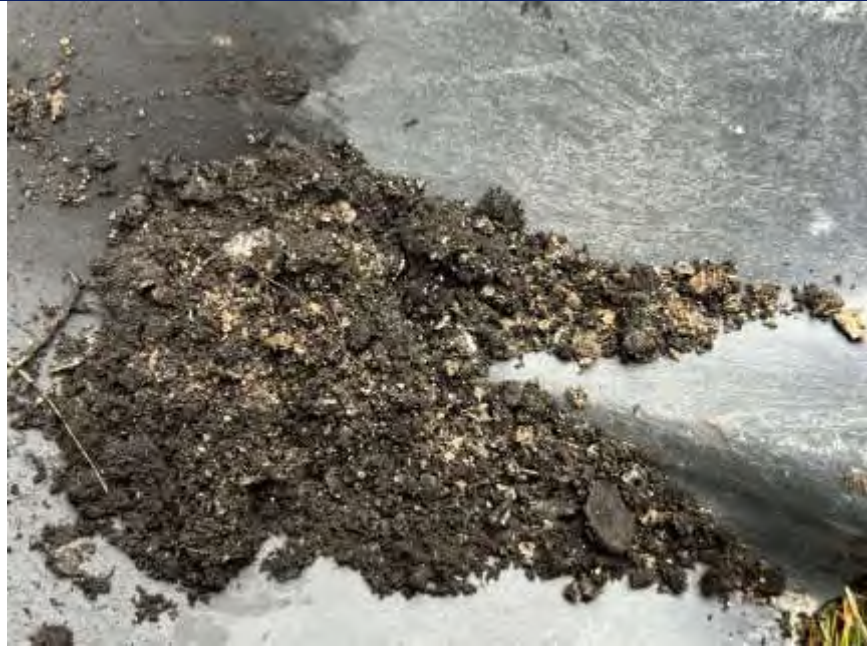
Photo 7: Observed native mineral soils (glacial till) intermixed with topsoil from hand dug test pit investigation.
