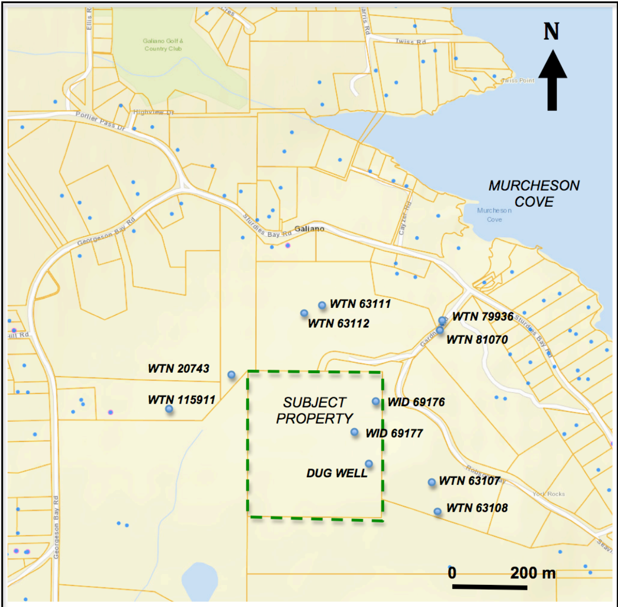
Figure 1. Location of subject property, pump tested wells (WID 69176 and WID 69177) and closest neighbouring wells. Basemap from Province of British Columbia (2023a).
