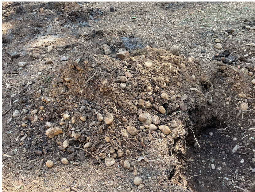
Photo. 4 Test Pit 2 with spoil pile. This is typical of the cobbly loamy sand soil in the area.
