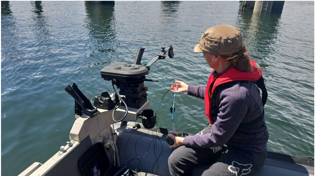
Photo 1-2. Showing the camera and downrigger ball setup used for the eelgrass surveys. Photo taken May 7, 2025.
