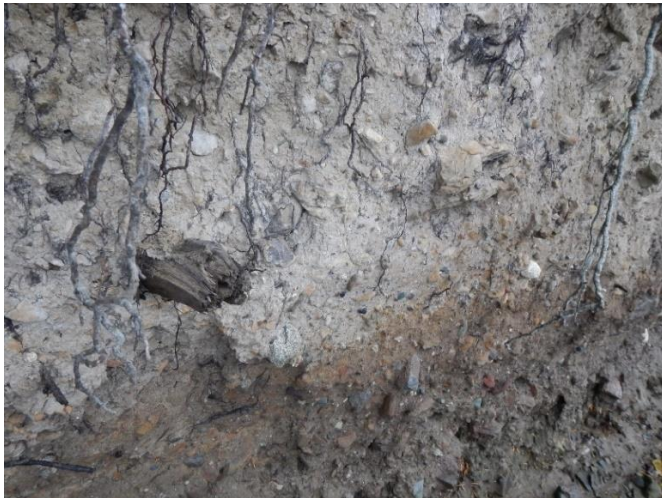
Figure 3. Close up photo of the cliff face. Note that many of the pebbles and cobble within the matrix are quite angular, which is not typical of a glacial till. Note also the large piece of wood protruding from the cliff; this wood did not appear to be a root but rather a trunk or branch. These observations point to excavated glacial till mixed with bedrock fragments that was pushed over an existing shoreline slope. The darker material to lower right may be the original till deposit at the site (photo collected to the west of the Anson Rd right-of-way).
