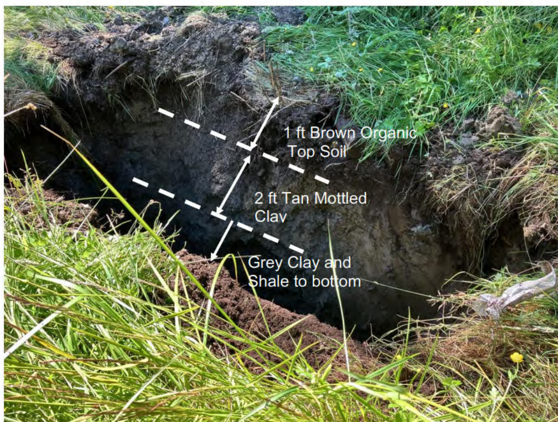
Photo 2. Exposed upper portion of soils in excavation for monitor well, June 30, 2025.
