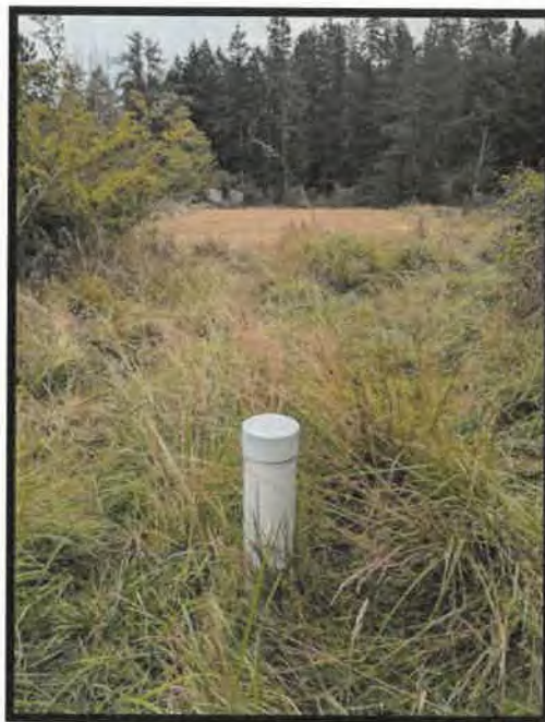
Photo 23: PVC stickup for newly established groundwater monitoring well.
