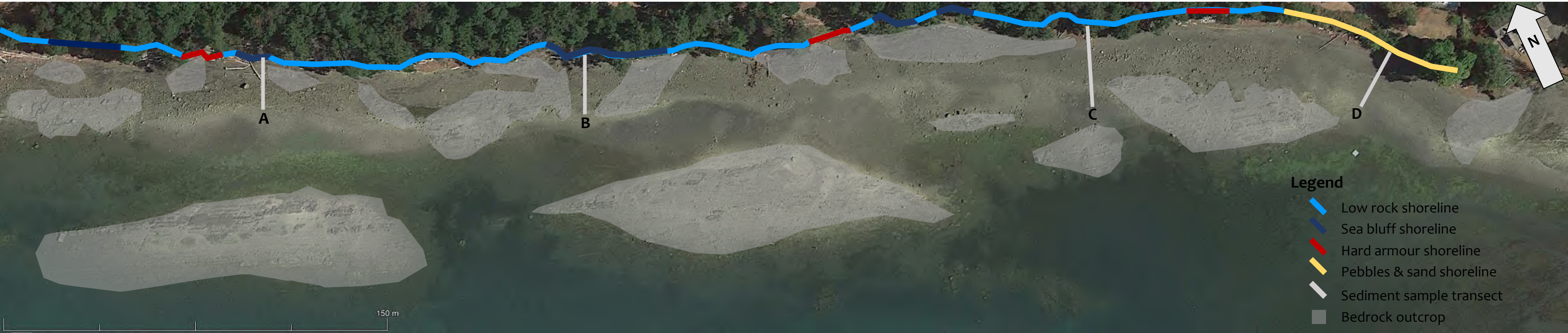
Figure 3. Shoreline types, sediment transects and bedrock outcroppings
