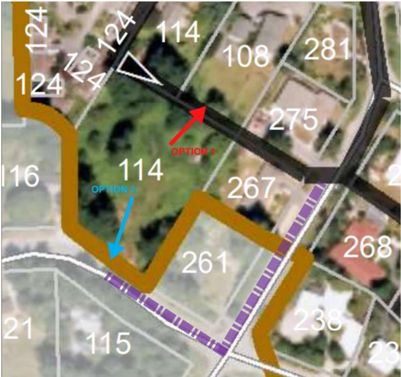
Figure 7: Options for connection to sewer system. Option 1 would require a cut across a Riparian Area, option 2 requires additional sewer infrastructure (in purple dashed line).
