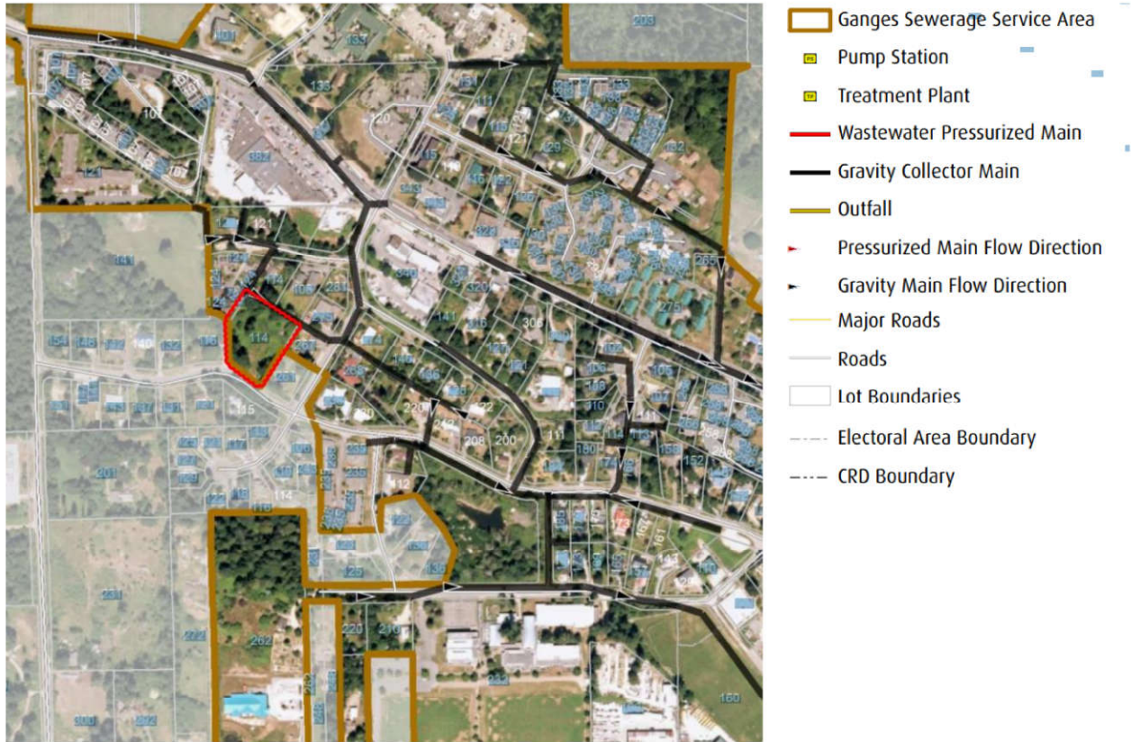
Figure 6: Location of CRD Sewer infrastructure.
